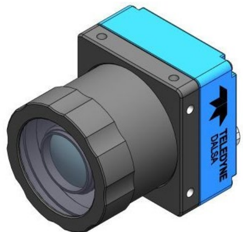
C-Mount Lens shown with Optional Cover
