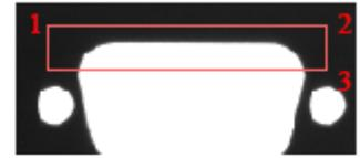
c. With the Caliper tool still selected, you can move or resize the rectangle region. Use the handles (solid green squares) at the top corners of the rectangle (first two click points) to adjust the angle or length of the region. Use the handle in the center of the rectangle's bottom edge to adjust the height.
