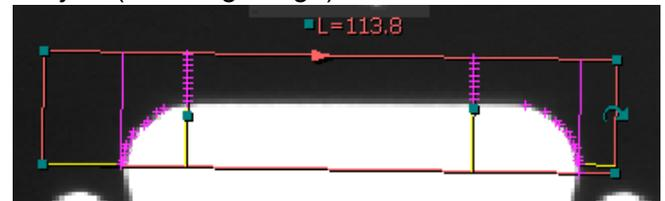
attached to the purple lines indicate the direction of the search, from the outside of the ROI toward the inside, or "Outside-in". The reported Length is the distance between the two purple lines.
