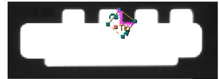
The pink crosses indicate the sample points, where the edges of the object were found. If the pink crosses are all on the edge of the search box, the tool properties (usually the direction) need to be adjusted for the correct measurement. The pink crosses should be on the edge of the object or point.
