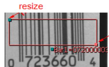
**Note:** The default "Orientation" or code direction is for horizontal codes from left to right, as shown (zero degrees). Codes at other angles (90, 180, 270) may not be recognized immediately with the default settings. The Details tab (Advanced settings) allows you to change this "orientation" to Automatic, or to a specific angle.
