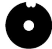
For this example, the good part has a score of 90, and the know defect has a score of 100. You will have to test your part to see what score a good part produces. You must lock the Tolerance and Perfect values so they do not change when you close or reopen the Match Tool Properties.
