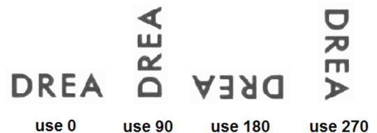
**Reduce** - when working with large characters, you can sub-sample the image at training and inspection time, to use less data, and run faster. Sub-sample should not be used with characters that have small or fine details.
