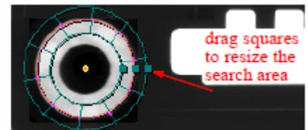
d. When you hover the cursor over the circle, the circle turns red, the location and intensity are displayed on the image, and a message appears telling you to “Right-click to edit.” Several radial lines appear at even spacing around the circle. These show the “sample points” for finding the edges of the circle.
