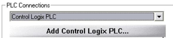
3. Set the PLC IP address to match your ControlLogix PLC, and then press the “Query Objs” button to get the PLC tags. Select (click) the tags your Solution will read from or write to, then click the “Add Variable” button.
