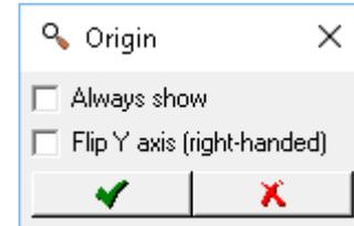
**Flip Y axis** - changes the direction of the Y axis and the direction of Rotation. Rotation is "positive" from the X axis to the Y axis. In the default setting, clockwise rotation is positive. In the "flip" setting, counter-clockwise rotation is positive.
